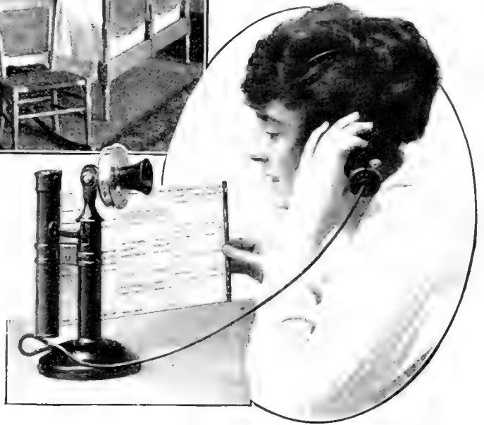
A Telephone Index Which Works on the Principle of a Roller Shade Has Been Put on the Market by a Boston Manufacturer. It Consists of a Coiled Spring in a Tubular Metal Case, Which is Clamped to the Pedestal of a Desk Telephone, and a Roll of Paper Ruled Off Most Conveniently
